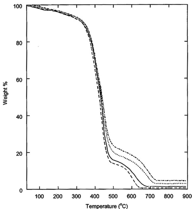
Fig. 6. Weight loss versus temperature as a function of component A, %: (---) Control, (—) IOHC1, (···) IOHC3, (- - -) IOHC4.
