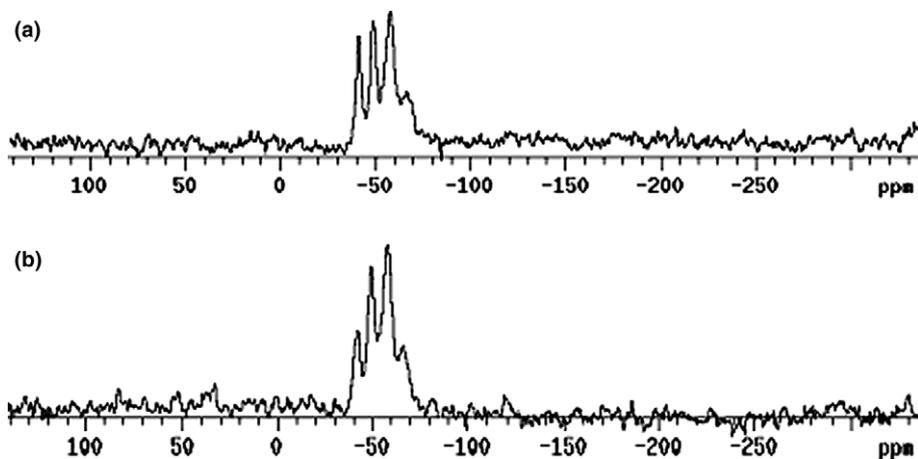
Fig. 3. Solid state  $^{29}\text{Si}$  NMR spectrum for (a) IOHC2 and (b) IOHC4.
