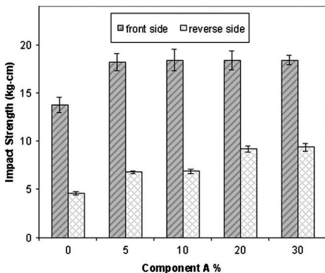
Fig. 5. The effect of amount of component A on the impact resistance of hybrid coatings.
