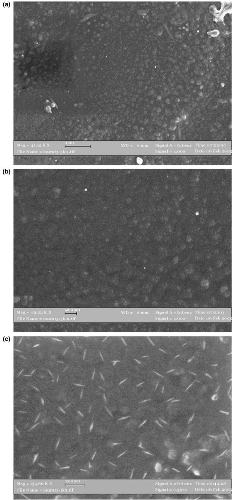
Fig. 7. SEM micrographs of hybrid coating with 30 wt% component A (IOHC4) at various magnification. The original magnifications and size bars are shown in the photomicrographs.
