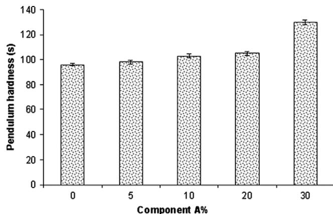
Fig. 4. The effect of amount of component A on the pendulum hardness of hybrid coatings.
