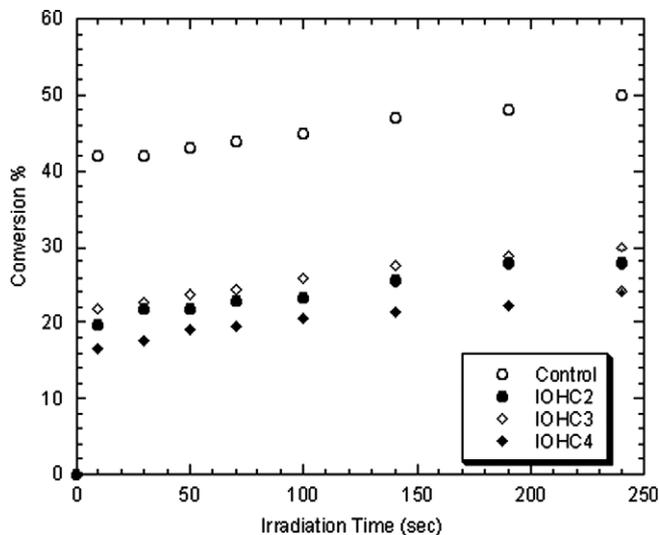
Fig. 2. RT-IR cure profiles showing the extent of double bond conversion versus time for hybrid films.
